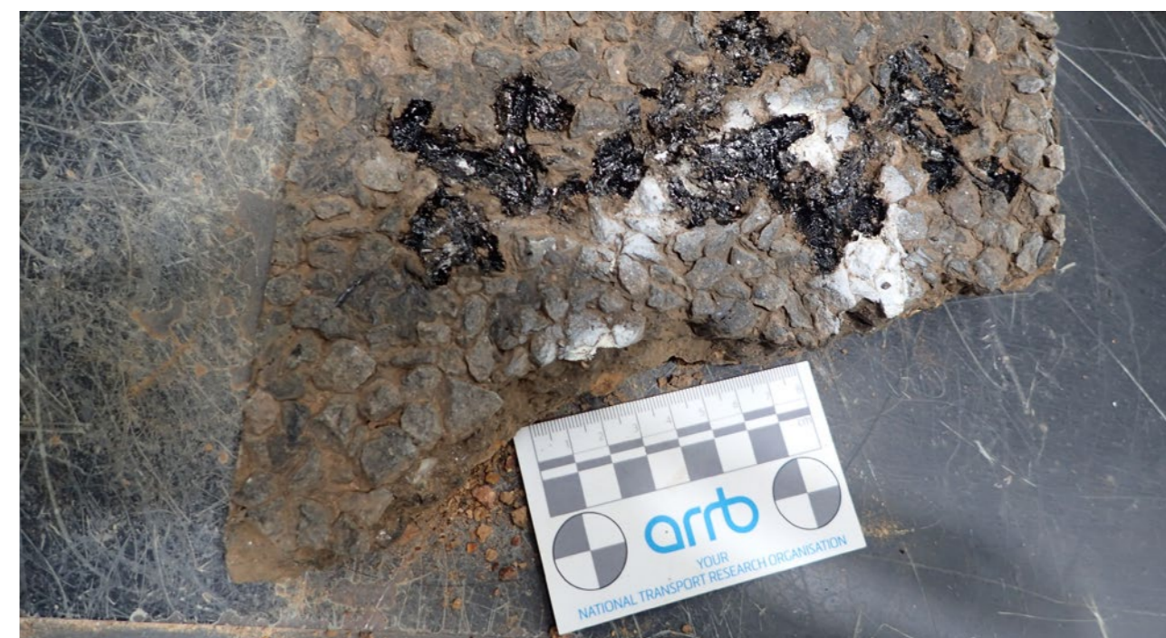
Figure 4 Field sampling of bitumen for in-field FTIR testing
