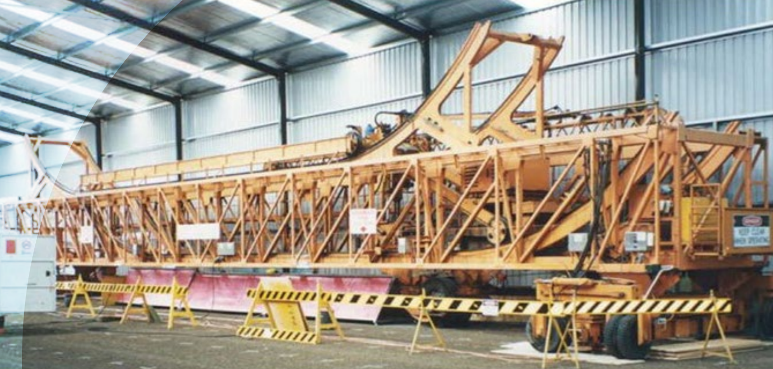
Figure 2 Accelerated Loading Facility (ALF) at Dandenong, Victoria.
