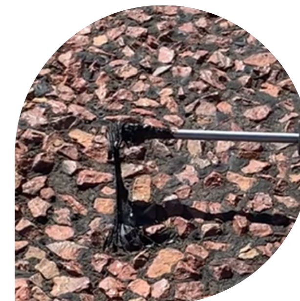
Figure 4 Field sampling of bitumen for in-field FTIR testing
