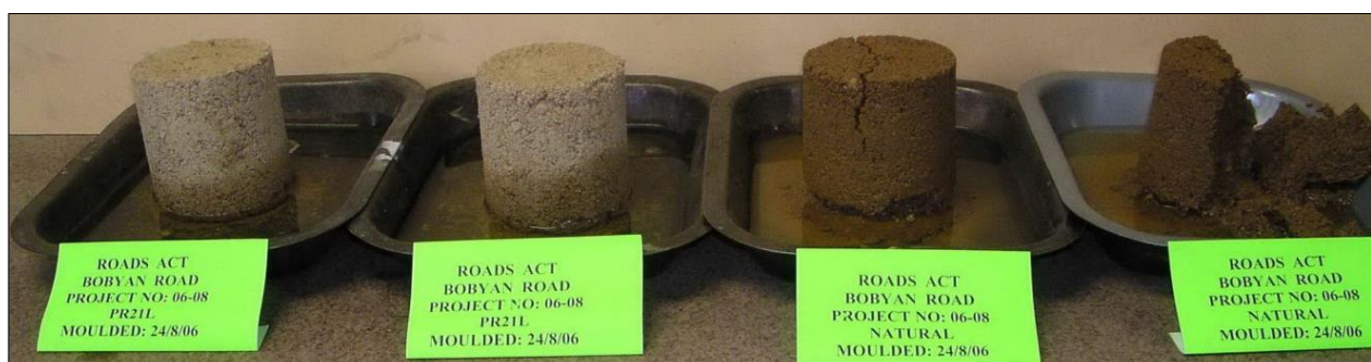
Figure 4.15: Vertical saturation test of chemical treated and untreated specimens
