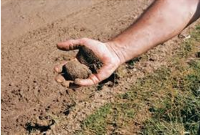
Figure 4.22: Simple field test for moisture content
