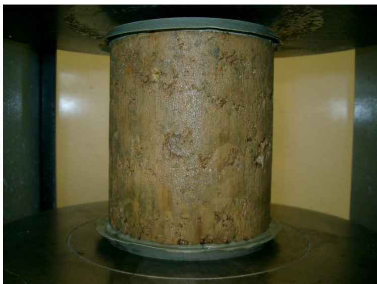
Figure 3.25: Unconfined compressive strength test apparatus and prepared sample
