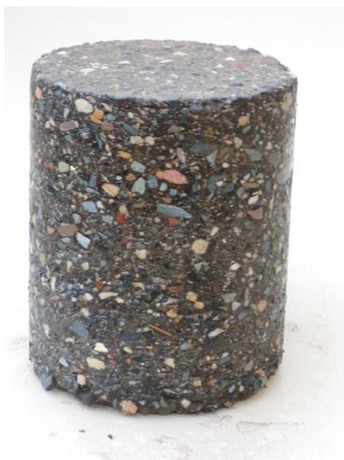
Figure 3.12: Bitumen stabilised basecourse with recycled aggregate
