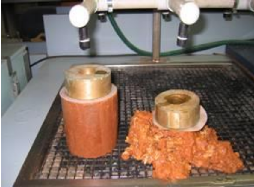
Figure 4.16: Strength test of chemical treated and untreated saturated specimens
