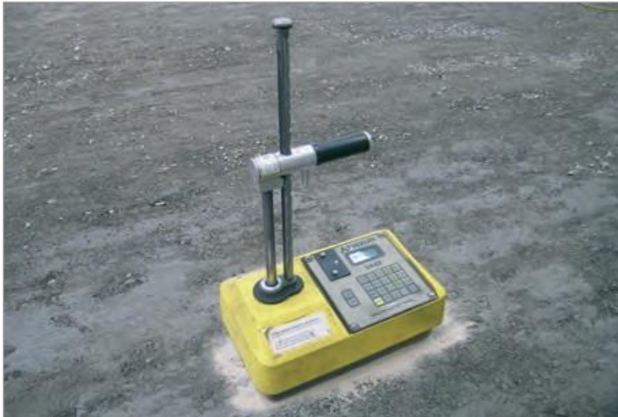
Figure 4.19: Nuclear density gauge
