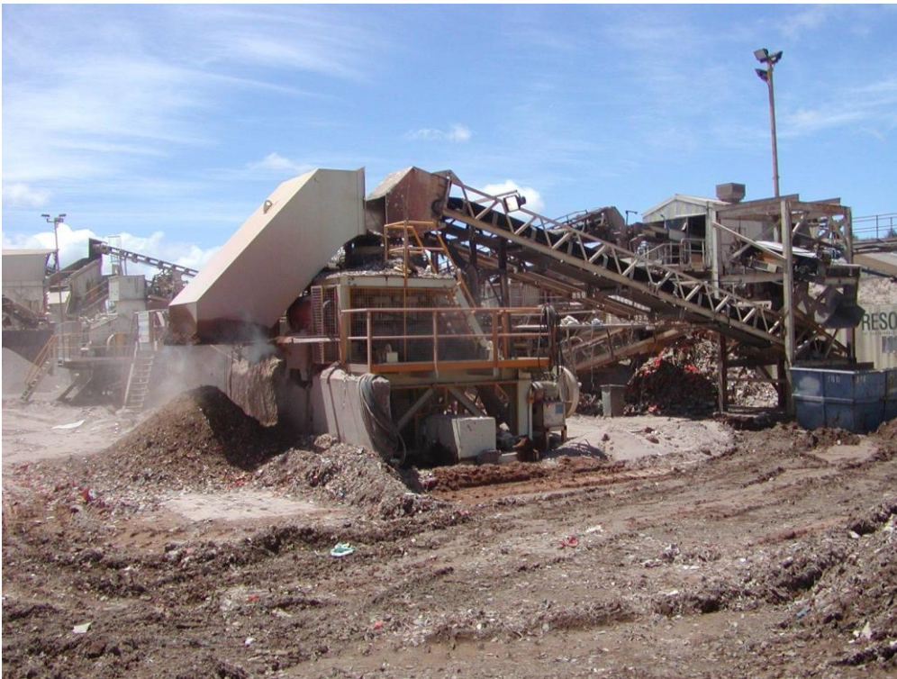
Figure 3.9: Recycling plant processing demolition waste
