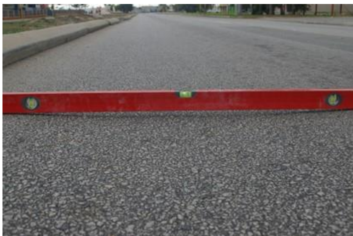
Figure 2.8: Manual measurement of rutting
