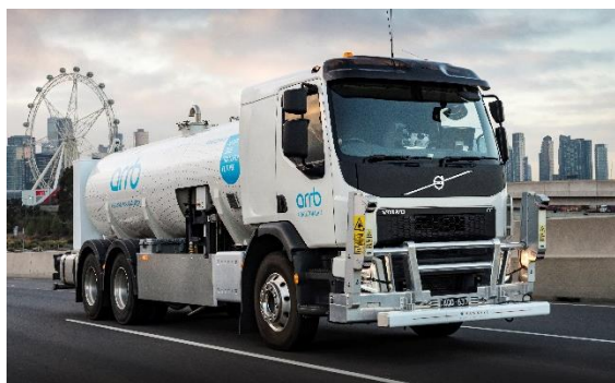
Figure 5.31: Intelligent safe surface assessment vehicle (iSSAVe)
