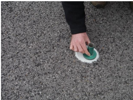
Figure 5.29: Sand patch testing (texture)
