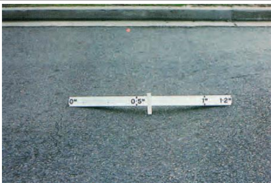
Figure 5.10: Depression/heave – depressions or bulges in the road surface
