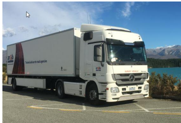
Figure 5.30: Travel speed deflectometer (iPAVe)
