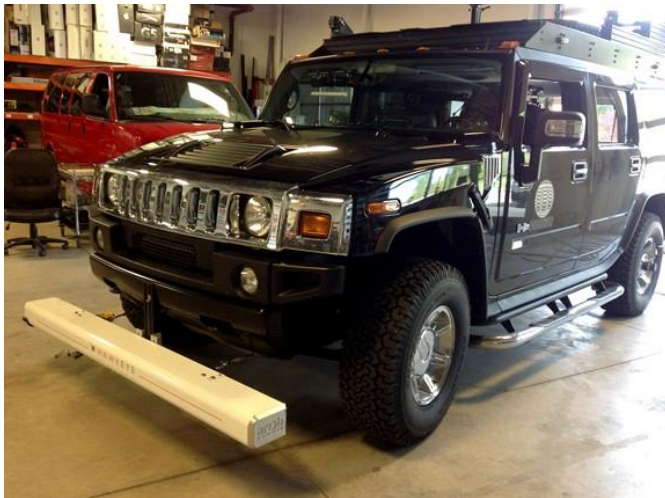
Figure 2.7: Inertial laser profilometer
