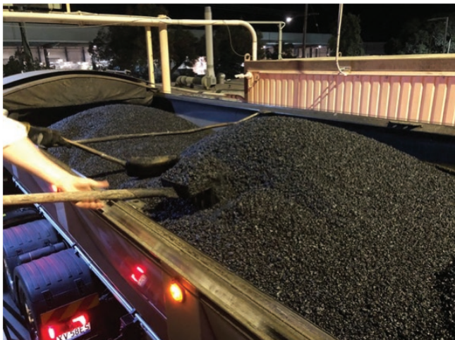
Figure 4: Collecting crumb rubber asphalt samples
