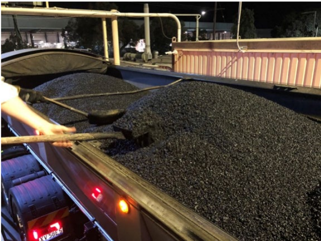
Figure 4: Collecting crumb rubber asphalt samples
