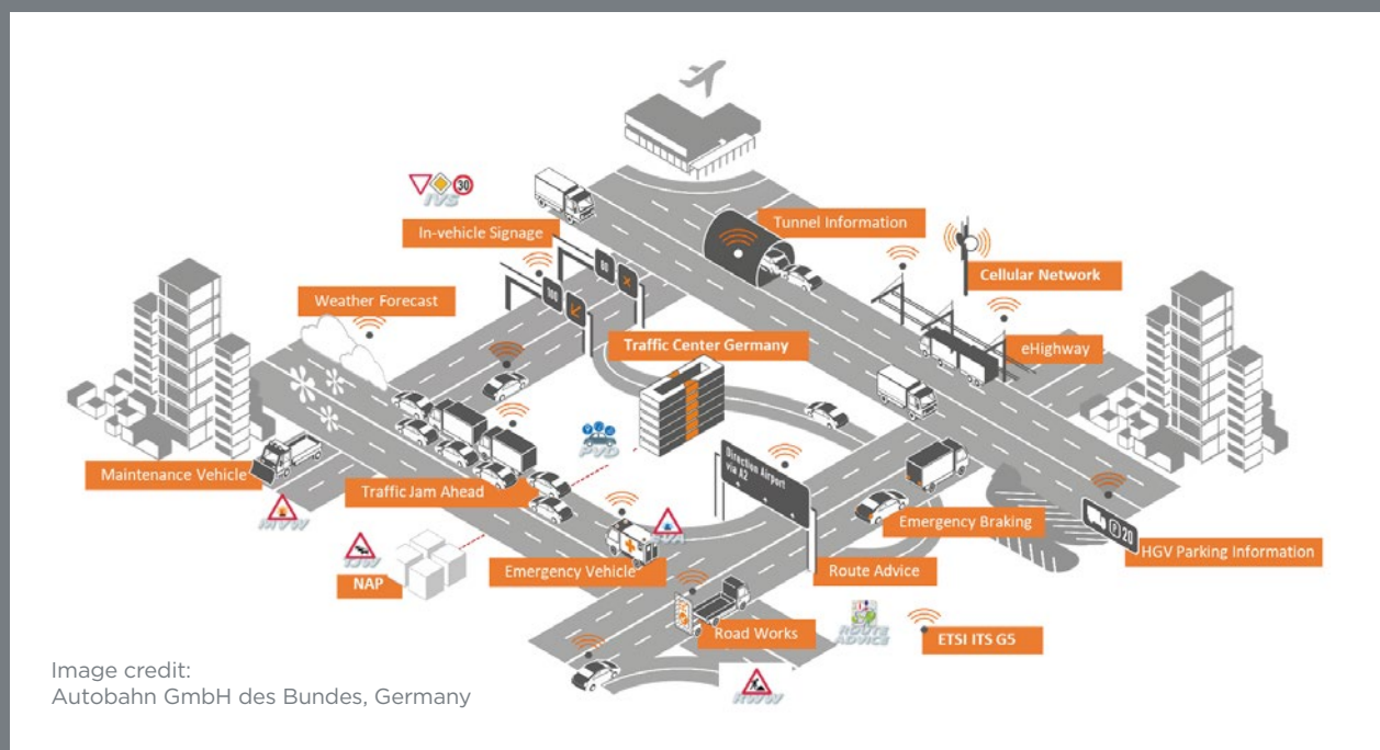
Figure 2: C-ITS AT A GLANCE, AUTOBAHN GMBH
